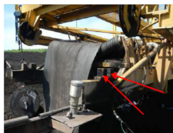
b) Damage that occurred on the carrying structure of the drum (left side);
