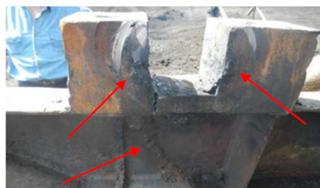
f) Damage and a crack at the carrying structure of an embedding of the stacker conveyor rejecting drum
