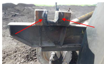
d) Damage at the structure of an embedding of the stacker conveyor rejecting drum – detail;
