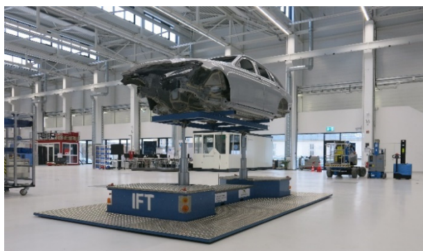
Figure 4. Prototype of the Mobile Assembly Island
