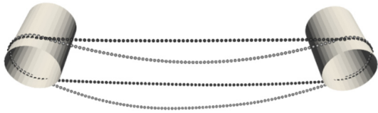
Figure 17: high and low tensioned particle chains on two pulleys, shown simultaneously
