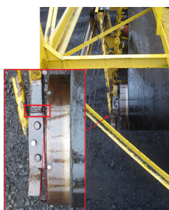
a) Appearance of the rejecting component of the stacker and of the last repair carried out in the area of the damage that occurred at the carrying structure of the drum;
