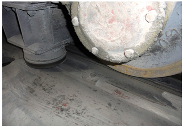
Figure 4. Wheel of a crane with a rail and a crane rail clip
