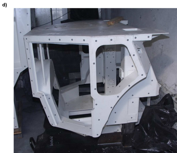
Figure 8. Sampling point for strain and acceleration measurements, points 1-3 – strain gauges, points 4-9 - accelerometers; a – points 2, 3, 7, b – points 1, 4, c – points 1-5, 7, 8, d – protective structure (side view)
