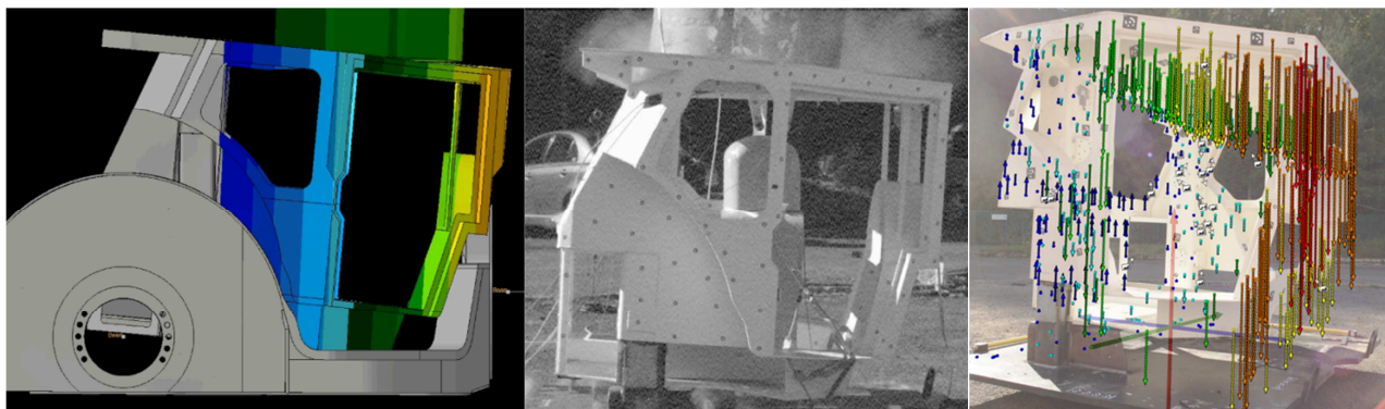
Figure 10. Overview of the methods measuring the deflection of the protective structure
