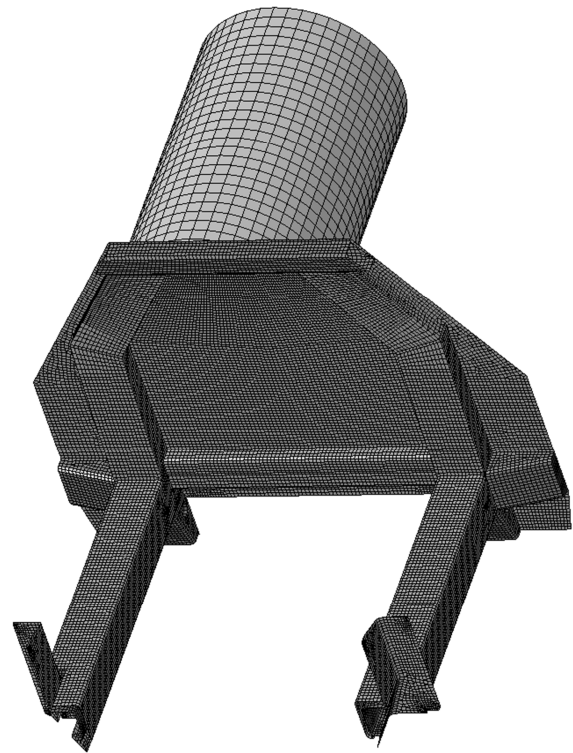
Figure 2. Discrete model of the cab (a) and assembly with platform and falling mass (b)
