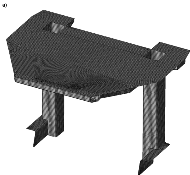
Figure 1. Geometrical model of the cab (a) and assembly with platform and falling mass (b)
