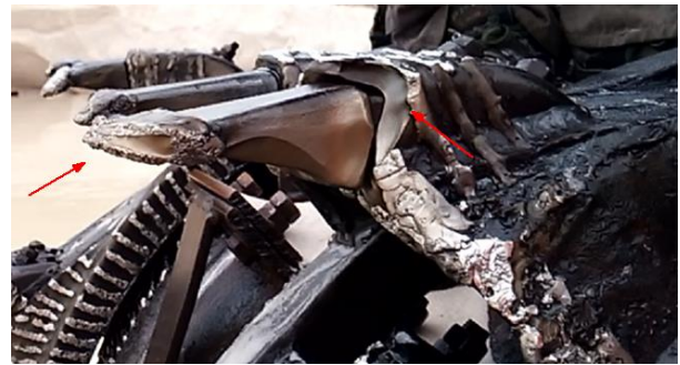
Figure 3. Unequal wear of teeth and bucket wheel wear areas
