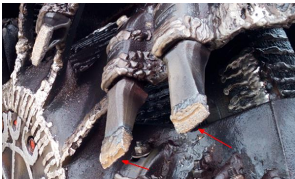
Figure 2. Typical wear of cutting teeth
