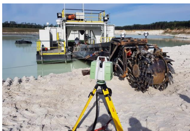
Fig. 3. Scanning the cutting tool geometry
