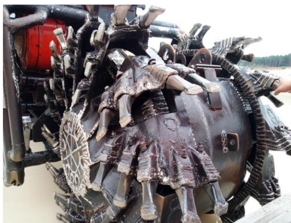
Fig. 2. Cutterhead of the dredger
